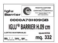
A lebel with the following informations: product's name and code, quantity, Certificate of the Environmental Compatibility, date of production, shift of production, n° of the worker, production line batch.
